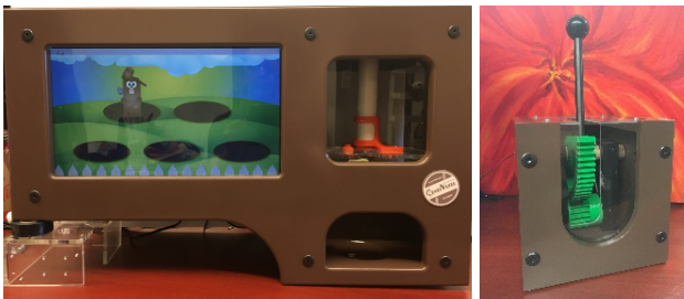
Figure 2. The Centivizer System (first prototype) with Whack-a-Mole cognitive game displayed (left side, left image) and nickel dispenser (right side, left image). An arm strengthening lever is also shown (right image).
