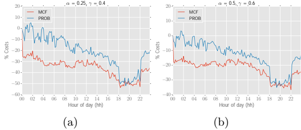
Figure 6: Percentage of cost savings w.r.t. NoForwarding on a daily scale, over the first day of the test query log for (a) \alpha = 0.25, \gamma = 0.4 and (b) \alpha = 0.5, \gamma = 0.6 .
