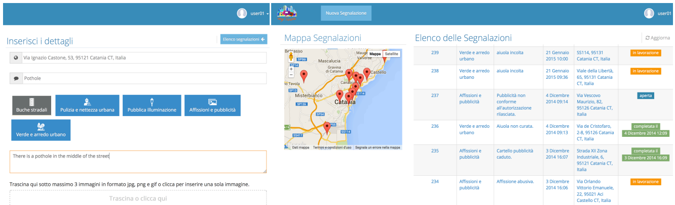
Figure 3: Some views on the front office web application. On the left, the form for the insertion of a new fault report is shown. On the right, the interface with the list of fault reports is shown.
