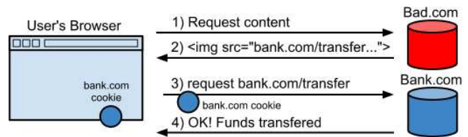
Figure 2: An example CSRF attack. When the user visits the adversary’s page, the HTTP reply (step 2) includes code that causes the user’s browser to make a request to bank.com (and attach bank.com ’s cookie). Bank.com erroneously treats this request as legitimate since it has the user’s cookie.
