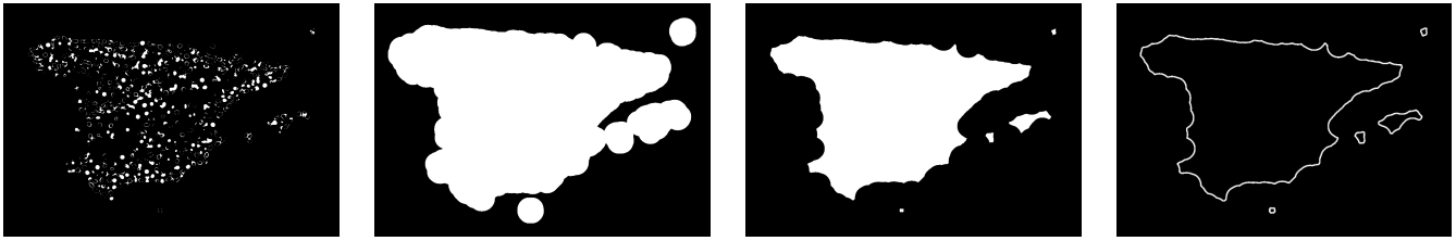
Figure 2: Region generation given a binary representation of the label Spain. We first fill all outer contours (left) and then smooth and connect disjoint areas by applying a morphological closing operation that first dilates (middle-left) and then erodes (middle-right) the binary representation, after which the contours are traced (right) to extract the characteristic regions. Here, the label was also prominently used on the Balearic islands (an archipelago of Spain), Melilla (an exclave of Spain) and in a small area in France, causing regions to emerge there as well.
