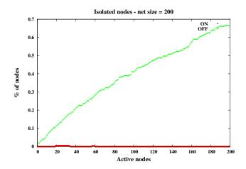
Figure 12: Amount of isolated nodes during a simulation; progressive node failures – clustered network;  $\gamma = 0.1, \omega = 0.1$ ; 200 nodes, 4 clusters (on average, there are  $4\omega$  inter-cluster links)
