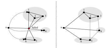
Figure 1: Reconfiguration at n after a node failure
