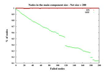
Figure 11: Main component size during a simulation; progressive node failures – clustered network;  $\gamma = 0.1, \omega = 0.1$ ; 200 nodes, 4 clusters (on average, there are  $4\omega$  inter-cluster links)
