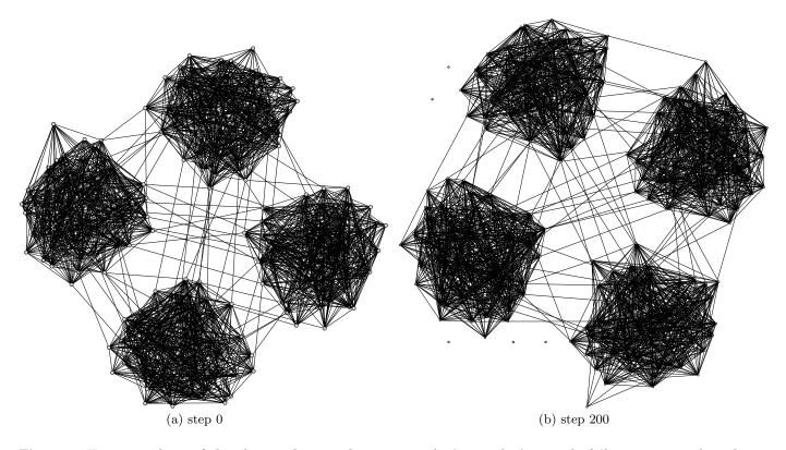
Figure 4: Two snapshots of the clustered network structure during evolution; node failure rate equal to the node join rate; 200 nodes, 4 clusters,  $\gamma = 0.5$ ,  $\omega = 0.2$  (hence on average there are  $4\omega = 10$  inter-cluster links)
