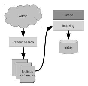
Figure 3: Indexing process
