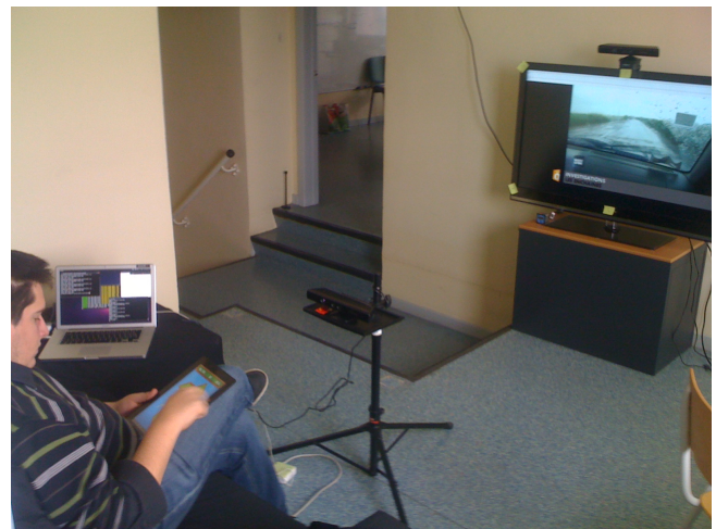
Figure 1: Setup of the experiment with the user playing a puzzle game on the second screen while a TV show is broadcast on the main screen. The camera in the middle of the scene tracks head movements (looking at the main screen or not).
