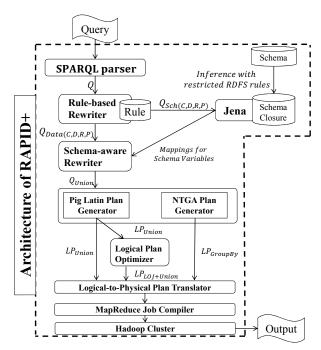
Figure 3: The architecture and Dataflow of RAPID+.
