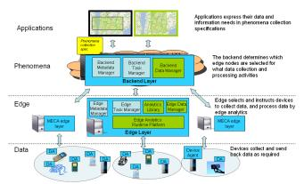
Figure 1: The three-layer architecture and components in MECA.
