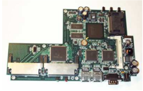
Figure 2: The Soekris net4521 single board computer
