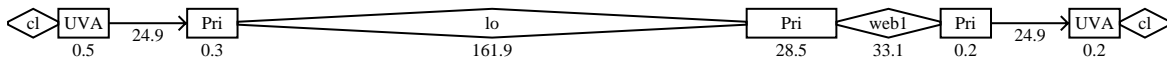
Figure 12: Linking algorithm output for a CoDeeN miss path with DNS lookup, delays in ms.
