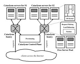
Figure 1: The Cataclysm Hosting Platform Architecture.
