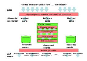
Figure 2: Processing stages in Deltarser for SAX.
