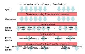
Figure 1: Processing stages in normal XML parsers for SAX.
