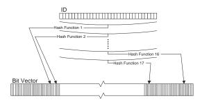
Figure 3: The classical Bloom Filters. The ID is 32 bits long, and 17 hash functions are used.
