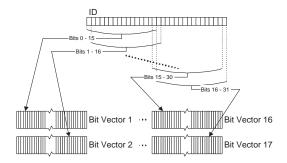
Figure 2: The overlapping bit-substrings solution. The ID is 32 bits long, and 17 bit vectors is of length  $2^{16}$  bits are kept.
