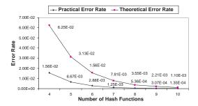
Figure 6: Comparing the Theoretical and the Practical Error Rates of Bloom Filters for Duplicate Detection on Jumping Window Using a Synthetic Click Stream
