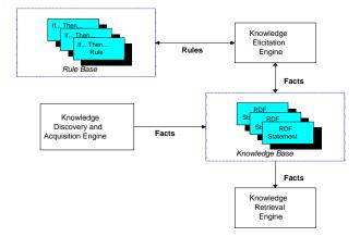
Figure 2 : System Architecture of the DSIC
