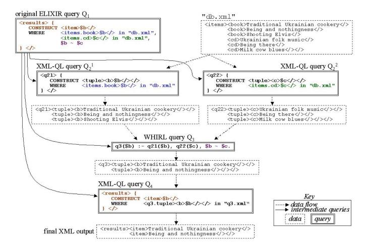
Figure 1: The ELIXIR query processor efficiently generates an answer to a query  $Q_1$  ("find books and CDs with similar titles") by rewriting  $Q_1$  into a series of XML-QL queries  $Q_2^i$ , a WHIRL query  $Q_3$ , and a final XML-QL query  $Q_4$ . Color indicates which parts of  $Q_B$  are used to generate the intermediate queries.
