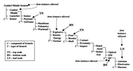
Figure 1 - Sample ontology showing a mixture of type-of and composed-of nodes
