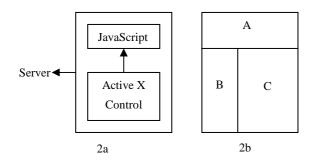
Figure 2. 2a shows the architecture of the client, 2b shows the appearance of the client to a user of the system.
