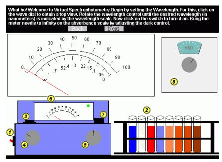
Figure 4. Screen snapshot of the spectrophotometry virtual laboratory. ① on/off switch, ② rack with test tubes with solutions, ③ sample holder for the test tube, ④ zero control dial, ⑤ light control dial, ⑥ meter with needle and pilot light (magnified view shown on top), ② wavelength control dial for setting the color of the illumination light, ⑧ magnified top view of the wavelength dial.
