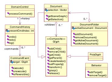
Figure 2. Domain class diagram of a generalized editor.
