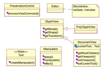
Figure 3. Presentation class diagram of a generalized editor.
