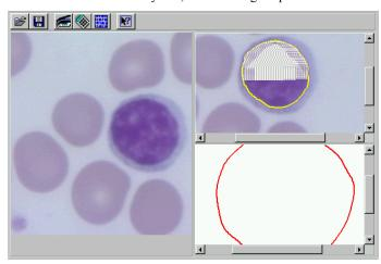
Figure 7. Screen snapshot of the virtual microscope lab. The original image taken from a microscope is shown on the left. The user selects a region of interest by a pen-based gesture and the system automatically segments the image and extracts various other features [3].
